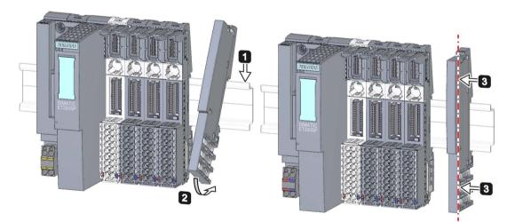
Figure 4-6 Installing the server module
