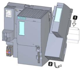
Figure 4-3 Installing CM DP
