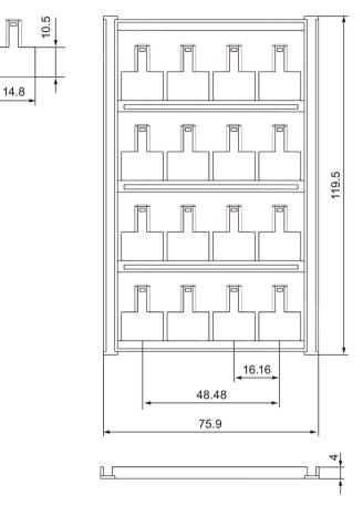
Figure A-3 Dimensional diagram of reference identification label and sheet
