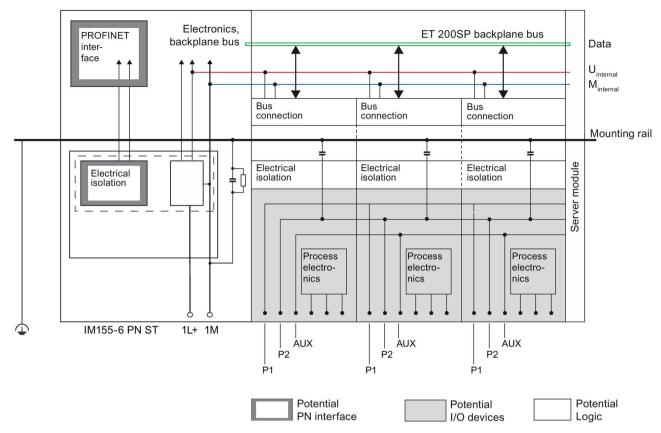
Figure 5-3 Electrical relationships for ET 200SP with interface module (using IM 155-6 PN ST as an example)
