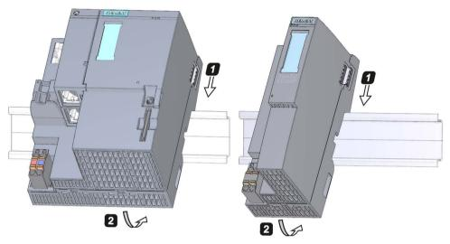
Figure 4-2 Mounting the CPU/interface module
