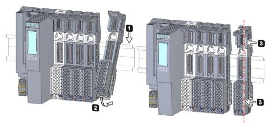
Figure 4-4 Installing a BaseUnit
