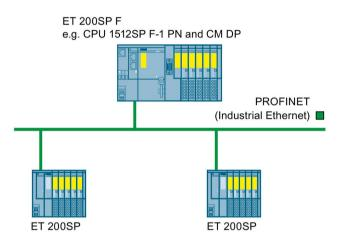
Figure 2-3 Fail-safe SIMATIC Safety automation system (sample configuration)
