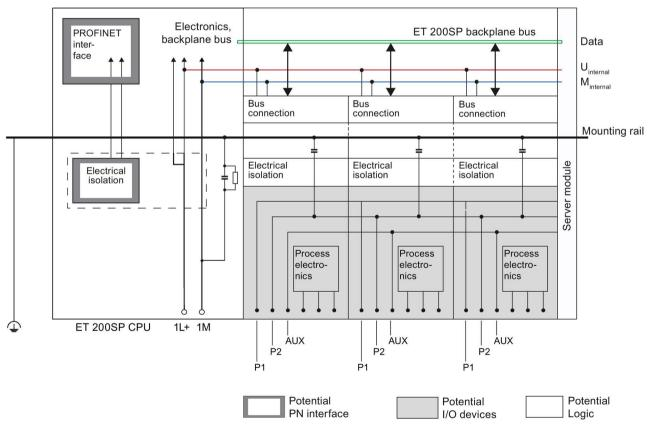
Figure 5-2 Electrical relationships for ET 200SP with CPU
