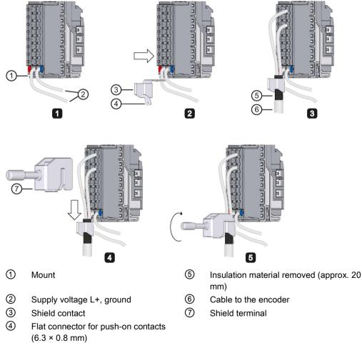
Figure 5-7 Mounting the shield contact
