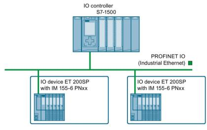
Figure 10-3 ET 200SP as an IO device
