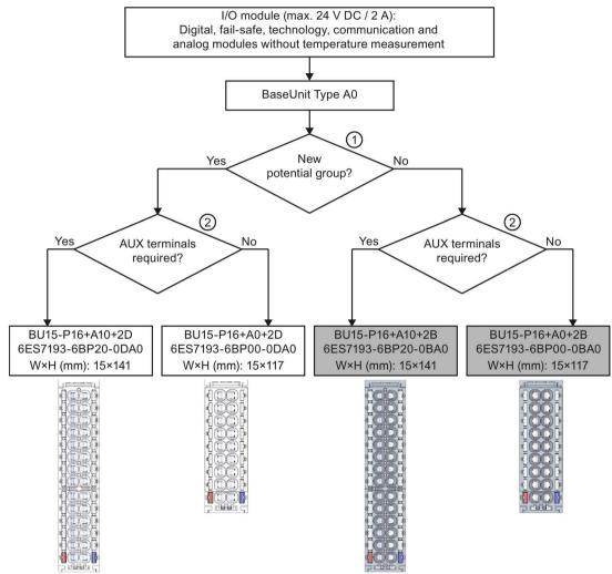
① Light-colored BaseUnit: Configuration of a new potential group, electrical isolation from adjacent module on the left. The first BaseUnit of the ET 200SP is usually a light-colored BaseUnit for feeding the supply voltage L+.
