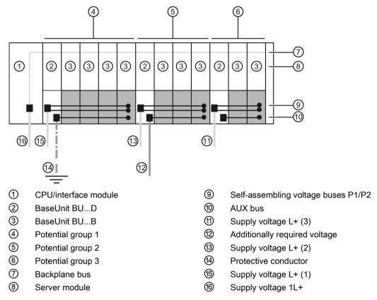
Figure 3-3 Placing the BaseUnits
