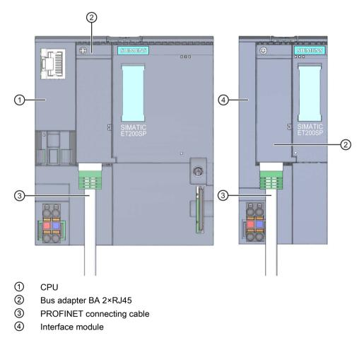
Figure 5-10 Connecting BusAdapter BA 2×RJ45 to the CPU/interface module
