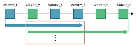
Figure 7-2 Parallel processing of the asynchronous instruction WRREC
